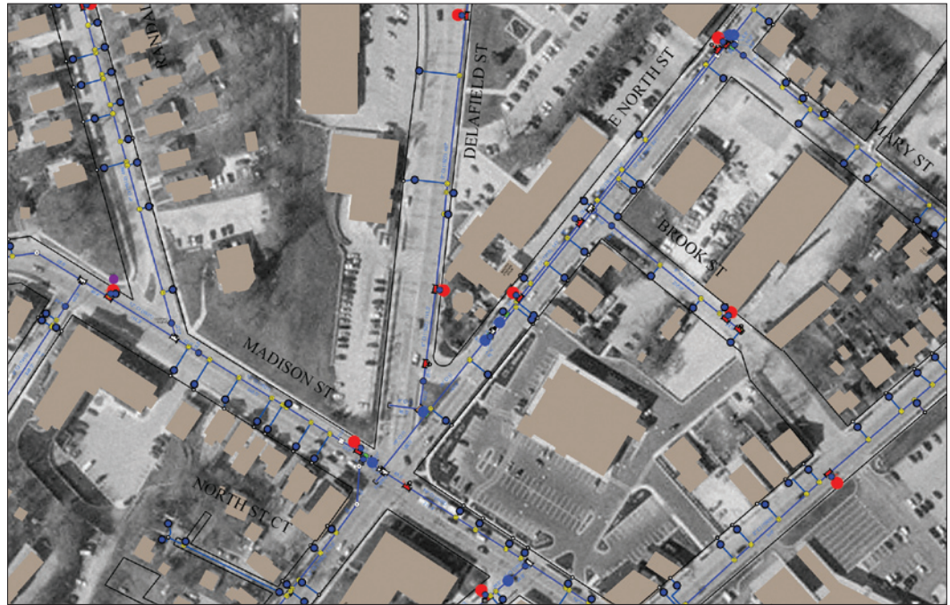
This GIS image of the Waukesha Water Utility's water distribution system shows the complexity of the system and the connections to hydrants, valves, and services.
